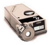
The low cost ExChek single sensor gas detector is designed to continuously monitor explosive range (0-100% LEL) combustible gas. Two modes of operation provide the right amount of information for users with different skill levels. In the Text Only ("OK") mode, the ExChek functions as a simple "Go/No Go" gas detector. The top-mounted LCD shows an "OK" message as long as conditions are safe. If an alarm condition occurs the audible and visual alarms are activated and readings are given in numbers.
