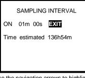
3. Use the navigation arrows to highlight the time interval (usually in minutes).
