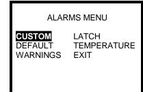
2. Use the navigation arrows to highlight CUSTOM and press the MODE button. The current alarm settings screen will then be shown.
