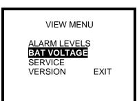
2. Use the navigation arrows to highlight BAT VOLTAGE and press the MODE button. The battery voltage screen will be shown.
