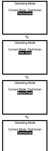
3. Once the preferred operating mode is highlighted, confirm the selection by pressing the MODE button.
