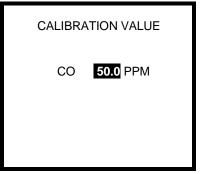
5. Use the up and down navigation arrows to adjust the calibration value.
