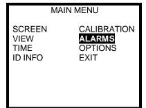
2. Use the navigation arrows to highlight ALARMS and press the MODE button. The Alarms Menu will then be shown.
