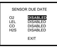
3. To enable (or disable) the service due setting for an individual sensor, use the up and down navigation arrows to highlight the setting adjacent to the sensor, and then press the right or left navigation arrow once.
