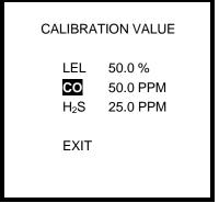
4. Press the MODE button to confirm the selection. The concentration will then be highlighted.
