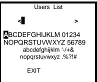
8. With the appropriate character highlighted, press the MODE button to enter the highlighted character into the highlighted space. The cursor will automatically move to the next available space.
