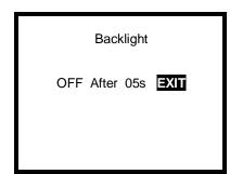
2. Use the right and left navigation arrows to highlight the time interval in seconds.
