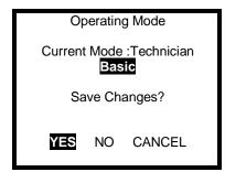
4. Press the MODE button with YES highlighted to accept the new operating mode
