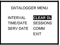
2. Use the navigation arrows to highlight CLEAR DL and press the MODE button.
