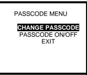
2. Use the up navigation arrow to highlight CHANGE PASSCODE and press the MODE button. The new passcode screen will then be shown:
