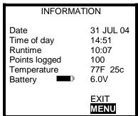
3. Press the down navigation arrow once to highlight MENU and press MODE button to enter the Main Menu.
