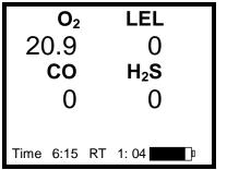
Current gas level screen in Basic, Basic/Peak and Technician Modes, no alarms present.
