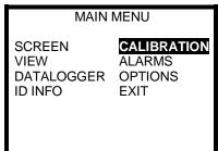
6. Use the navigation arrows to highlight CALIBRATION and press the MODE button.
