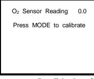
7. The oxygen reading will drop immediately and should approach a reading of 0.0 percent oxygen, but may not actually stabilize at 0.0. Press the MODE button when the oxygen reading stabilizes to calibrate the sensor.
