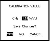
8. Press the MODE button with YES highlighted to save the new settings.
