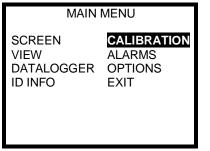
3. Use the navigation arrows to select CALIBRATION and press the MODE button.
