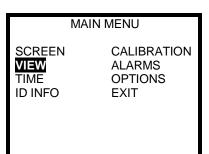
2. Use the navigation arrows to highlight VIEW and press the MODE button. The View Menu will then be shown.
