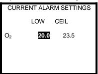
6. When the alarm adjustment for a particular sensor is complete, press the MODE button to enter the new setting.
