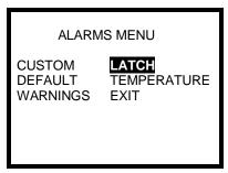
2. Use the navigation arrows to highlight LATCH and press the MODE button. The alarm latch settings screen will then appear.
