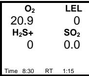
Current gas readings screens with CO Plus sensor; calibration gas setting set to  $\ensuremath{\text{H}_2S}\xspace$
