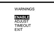
Use the up and down navigation arrows to highlight ENABLE and press the MODE button. The enabled or disabled setting for the warning alarms will be shown between WARNINGS and EXIT. Use the up and down navigation arrows to change the setting.
