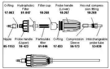
Figure 2.5.2. Cannonball3 sample draw probe.
