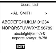
12. Press the MODE button with EXIT highlighted to return to the users list screen.
