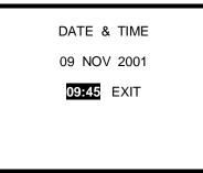
3. The right and left navigation arrows are used to move back and forth between the day, month, year, and time settings and the exit key. Once the time setting that needs to be adjusted is highlighted, the up and down navigation arrows are used to adjust the setting.
