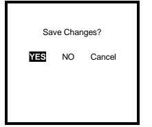
5 Press the MODE button with YES highlighted to save the new warning alarm setting.
