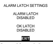
3. Use the up and down navigation arrows to select the ENABLED/DISABLED setting for the OK latch.
