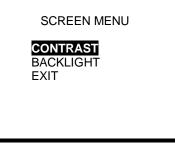
2. Use the up navigation arrow to highlight CONTRAST and press the MODE button.
