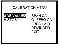
2. Use the navigation arrows to highlight GAS VALUES and press the MODE button.
