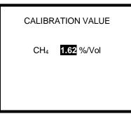
7. Once the appropriate calibration gas concentration is reached, press the MODE button to confirm the setting.
