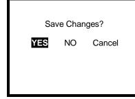
5. Press the MODE button with YES highlighted to confirm the new settings.
