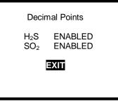
6. Once the appropriate decimal point settings have been entered, use the navigation arrows to highlight EXIT and press the MODE button to enter the new settings.
