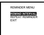
Use the navigation arrows to highlight "REMIND INTERVAL" and press the MODE button. The reminder interval will be shown as either "Every" with the number of days shown, or as "Never".
