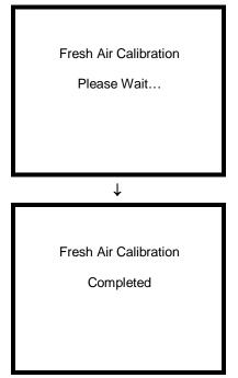
7. After the completion of the fresh air calibration the Cannonball3 will automatically return to the Main Menu.
