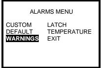
2. Use the navigation arrows to highlight WARNINGS and press the MODE button. The warning alarm settings screen will then be shown.
