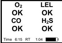
Current gas level screen in Text Only mode, no alarms present.
