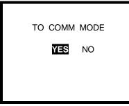
3. Press the MODE button with YES highlighted to enter communication mode and enable the IrDA port.
