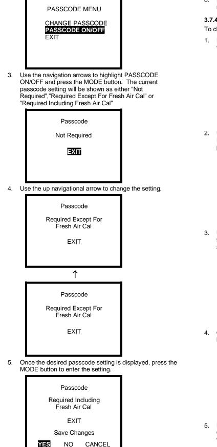
6. Press the MODE button with YES highlighted to save the new passcode setting.
