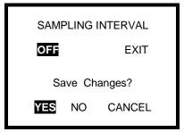
5. Press MODE with YES highlighted to save the new sampling interval setting.
