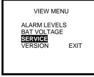
2. Use the navigation arrows to highlight SERVICE and press the MODE button. The service information screen will be shown.
