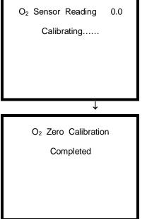
After the successful completion of the  $O_2$  zero calibration, the instrument will return to the Main Menu. Disconnect the calibration gas cylinder immediately.
