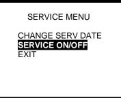
2. Use the up navigation arrows to highlight SERVICE ON/OFF and press the MODE button.
