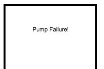
Following a pump test failure, the instrument will shut itself off. In the event of a pump failure, perform the following steps:
