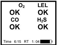
Current gas level screen in Text Only mode, no alarms present. If an alarm condition occurs the indication changes from "OK" to the numerical value, the LED alarm lights flash, and the audible alarm sounds.
