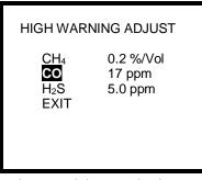
4. Use the up and down navigation arrows to highlight the alarm for adjustment and press the MODE button.
