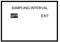
4. The up and down navigational arrows are used to toggle between ON and OFF. Press the MODE button with OFF highlighted.
