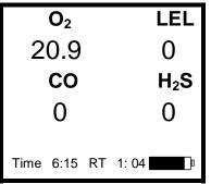
Current gas level screen in Basic, Basic/Peak and Technician Modes.
