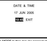
The MODE button may be pressed at any time to confirm 4. the new time settings.
