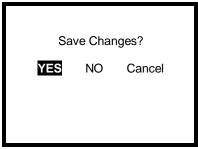
5. Press the MODE button with YES highlighted to save the new warning alarm setting.
