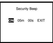
5. The interval setting will appear when the security beep is turned ON (as above). Use the right and left navigation arrows to highlight the interval if it requires adjustment.
