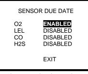
Once the sensor due date settings are enabled or disabled 4. as required, press the MODE button to enter the settings.
