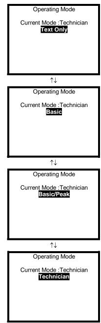
6. Once the preferred operating mode is highlighted, confirm the selection by pressing the MODE button.
