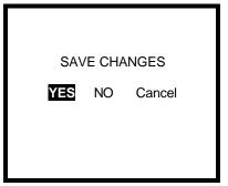
10. Press the MODE button with yes highlighted to save changes. Remove all fittings before turning the instrument back on and returning to normal operation.
