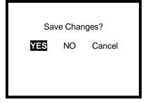
7. Press the mode button with YES highlighted to save the new decimal settings.
