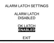
4. Use the left and right navigation arrows to toggle between ENABLED and DISABLED. Once the appropriate setting is reached, press the MODE button to confirm your selection.
