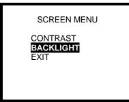
2. Use the up navigation arrow to highlight BACKLIGHT and press the MODE button.
