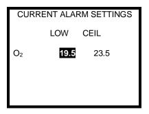
5. Use the right and left navigation arrows to select the specific alarm for modification. Once the specific alarm is selected, use the up and down navigation arrows to modify the current alarm setting.
