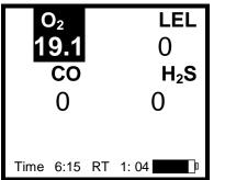
Current gas level screen in alarm condition in Basic, Basic/Peak and Technician Modes.
