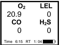
Current gas level screen in Basic, Basic/Peak and Technician modes with no alarms present.
