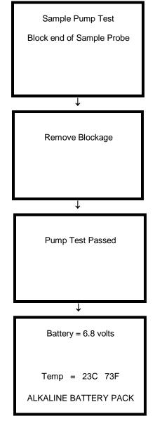
Note: If the sample pump test fails, see section 6.2.3. **WARNING** The accuracy of the Cannonball3 should be checked periodically with known concentration calibration gas. Failure to check accuracy can lead to inaccurate and potentially dangerous readings.
