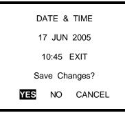
Press the MODE button with YES highlighted to confirm 5. the new time and date settings.
