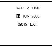
3. The right and left navigation arrows are used to move back and forth between the day, month, year, and time settings and the EXIT option. Once the time setting that needs to be adjusted is highlighted, the up and down navigation arrows are used to adjust the setting.
