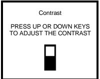
3. Adjust the contrast with the up and down navigation arrows. When the contrast reaches the desired level press the MODE button.
