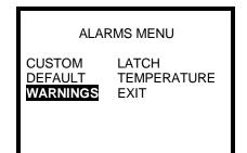
2. Use the navigation arrows to highlight WARNINGS and press the MODE button. The warning alarm settings screen will then be shown.
