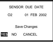
6. Press the MODE button with YES highlighted to confirm the new service due date settings.
