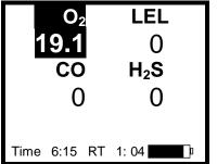
Current gas level screen in Basic, Basic/Peak and Technician Modes, alarm condition.
