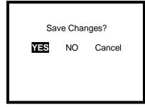
6. Press the MODE button with YES highlighted to save the new temperature alarm settings.
