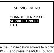
2. Use the up navigation arrows to highlight SERVICE ON/OFF and press the MODE button.
