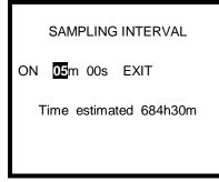
5. Once the sampling interval is adjusted, press the MODE button to enter the new interval.
