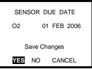
6. Press the MODE button with YES highlighted to confirm the new service due date settings.
