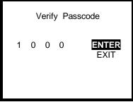
6. Press the MODE button with ENTER highlighted to confirm the new passcode.
