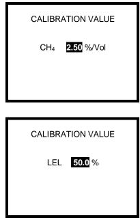
4. The right and left navigation arrows may be used to move back and forth between the calibration gas setting (LEL or CH<sub>4</sub>) and the calibration gas concentration. To change the calibration gas setting, press the left navigation arrow once to highlight LEL or CH<sub>4</sub>.
