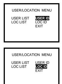
2. Press the MODE button to confirm the selection. The current user or location ID will then be shown.
