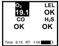
Text Only mode current gas level screen with alarm condition.
