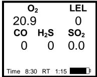
Current gas readings screen with Duo-Tox and  $\mbox{SO}_2$  toxic sensors installed.
