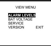
2. Use the navigation arrows to highlight ALARM LEVELS and press the MODE button. The current alarm settings screen will then be shown.
