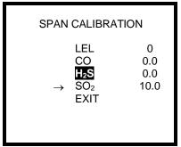
**WARNING** If using the calibration balloon and the calibration of more than one sensor is required, deflate the calibration balloon fully before filling it with new gas for subsequent calibrations. Failure to fully deflate the calibration balloon between calibrations may lead to inaccurate and potentially dangerous readings.
