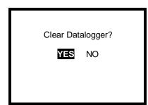
3. Press the MODE button with YES highlighted to clear the datalogger memory.
