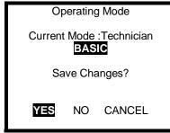
7. Press the MODE button with YES highlighted to save the new operating mode.
