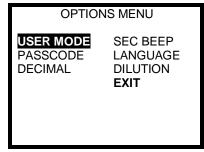
5. Use the navigations arrows to highlight USER MODE and press the MODE button. The up and down navigation arrows may then be used to toggle between operating modes.
