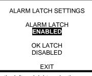
4. Use the left and right navigation arrows to toggle between ENABLED and DISABLED. Once the desired setting is reached, press the MODE button to confirm the selection.
