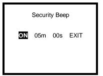
4. With ON or OFF highlighted, the up and down navigation arrows allow the user to toggle between security beep on and security beep off.
