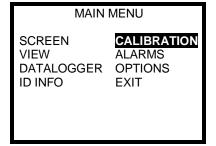
4. Use the navigation arrows to select CALIBRATION and then press the MODE button.
