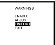
3. Use the up and down navigation arrows to highlight TIMEOUT and press the MODE button.
