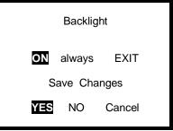
5. Press the mode button with YES highlighted to save the new backlight setting.
