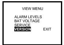
2. Use the navigation arrows to highlight VERSION and press the MODE button. The software version screen then be shown.
