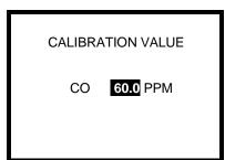
6. Once the concentration matches the value listed on the calibration gas cylinder, press the MODE button.
