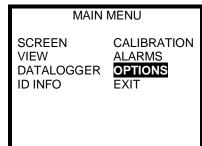
4. Press the up arrow once to highlight OPTIONS and press the MODE button to enter the Options Menu.
