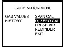
4. Use the navigation arrows to highlight O<sub>2</sub> ZERO CAL and press the MODE button.
