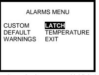
2. Use the navigation arrows to highlight LATCH and press the MODE button. The alarm latch settings screen will then be shown.
