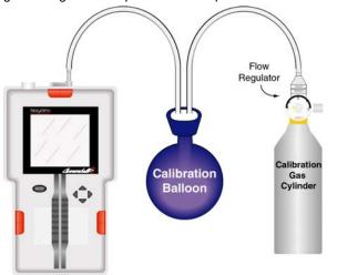
Cannonball3 with calibration balloon and calibration gas cylinder.
