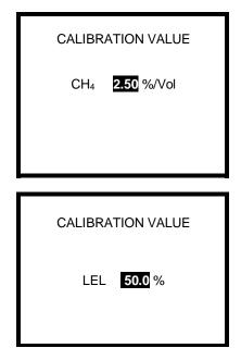
To change the concentration of LEL or CH<sub>4</sub> used in calibration, use the right navigation arrow to highlight the calibration gas concentration. With the concentration value highlighted, adjustments to the gas concentration may then be made using the up and down navigation arrows.
