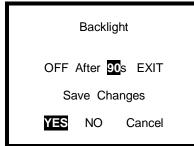
5. Press the mode button with YES highlighted to save the new interval setting.
