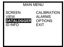
6. Use the navigation arrows to highlight DATALOGGER and press the MODE button.
