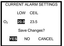
7. Press the MODE button with YES highlighted to save the new alarm settings. The instrument will then return to the current alarm settings screen.
