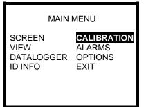
3. Use the navigation arrows to highlight CALIBRATION and press the MODE button.
