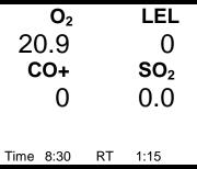
Current gas readings screens with CO Plus sensor; calibration gas setting set to CO.
