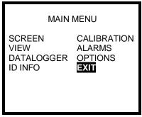
8. Press the MODE button with EXIT highlighted to return to the current gas readings screen.
