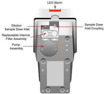
Figure 2.5.3 Bottom of lower case assembly.
