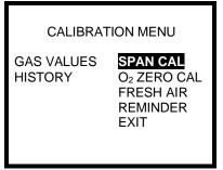
4. Use the navigation arrows to highlight SPAN CAL and press the MODE button.
