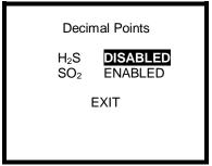
4. Press the left or right navigation button to change the toxic sensor's decimal point setting.
