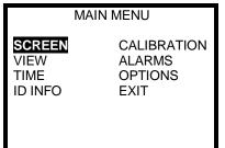
2. Use the navigation arrows highlight SCREEN and then press the MODE button to enter the Screen Menu.
