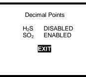
3. Use the up and down navigation arrows to highlight the enabled or disabled setting for the sensor whose decimal point setting requires adjustment.
