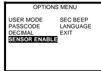
2. Use the navigation arrows to highlight SENSOR ENABLE and press the MODE button.
