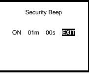
8. Press the MODE button with EXIT highlighted to exit the security beep option.
