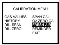
5. Use the navigation arrows to highlight FRESH AIR and press the MODE button.
