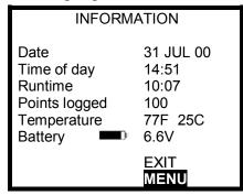
4. Press the down navigation arrow once to highlight MENU and press the MODE button.
