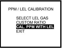
Use the up and down navigation arrows to highlight CAL PPM WITH LEL and press the MODE button. The following screen will be shown.
