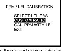
Use the up and down navigation arrows to highlight CUSTOM RATIO and press the MODE button
