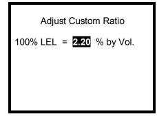
Use the up and down navigation arrows to adjust the ratio. Press the MODE button once the ratio is adjusted to the appropriate level.
