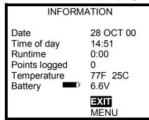
3. Hold down the left navigation arrow for 3 seconds or until EXIT appears and is highlighted.
