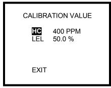
Press the MODE button once the appropriate concentration is highlighted. The concentration will then be highlighted.
