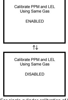
4. For single cylinder calibration of both the LEL and HC ranges, use the up and down navigation arrows to
