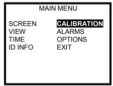
5. Use the navigation arrows to highlight CALIBRATION and press the MODE button. The Calibration Menu will then be shown. Note the addition of the PPM / LEL option.
