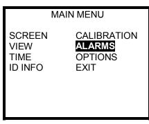
Use the navigation arrows to highlight ALARMS and press the MODE button. The Alarms Menu will then be shown.
