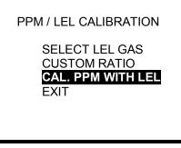
Use the up and down navigation arrows to highlight CAL PPM WITH LEL and press the MODE button. The following screen will be shown.
