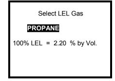
4. Use the up and down navigation arrows to scroll through the list of available gases until the specific gas that you expect to encounter in the PPM range is shown.
