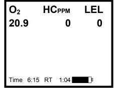
In the HCPPM mode, readings are displayed in 10-PPM increments from 0 – 10,000 PPM. At 10,000 PPM, the reading automatically switches to percent by volume (vol%) with 0.01 % resolution (100 PPM). The following table summarizes the display resolution across all ranges.
