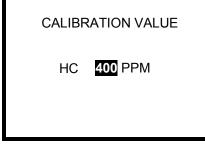
5. Use the up and down navigation arrows to adjust the calibration value.
