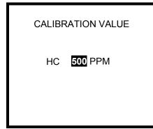
6. Once the concentration matches the value listed on the calibration gas cylinder, press the MODE button.
