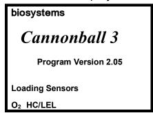
There are very few differences in the initial start up screens with the HC/LEL sensor installed versus the standard LEL sensor. One notable difference is the alarm display, which will show the distinct HC and LEL alarm setpoints.
